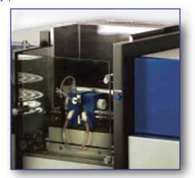
The instrument is equipped with a graphite Furnace Atomiser only. The graphite head is fixed into the optical path to maximise performance and eliminate drift.
